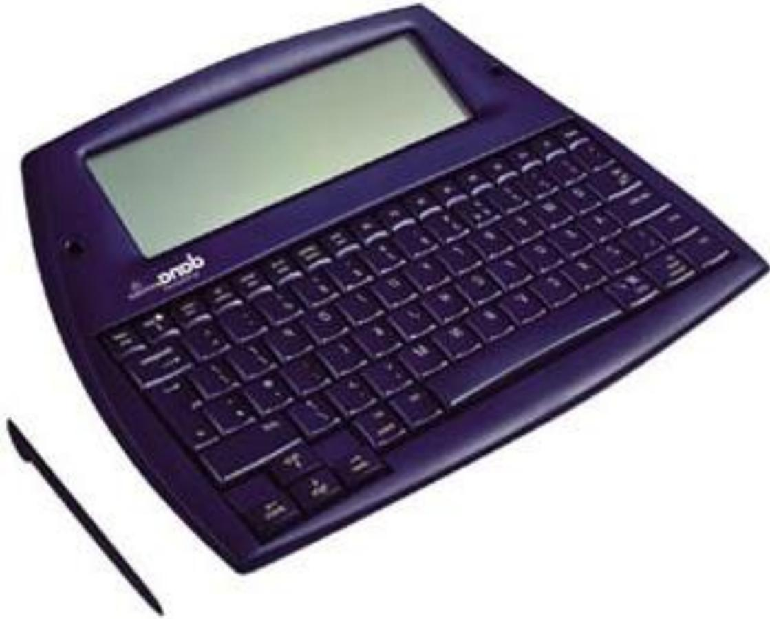
A **portable word processor**, often called a **portable keyboard**, is a lightweight device that is an alternative to using a laptop for writing. It can be easily transported from class to class and between home and school.
